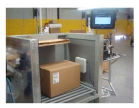
Our latest design comes with a touch-screen PC for operator input. We include a fixed RFID reader and an optional RFID printer for case-level printing. You may also choose an audio mode and larger fonts.
